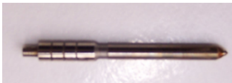
Figure 1 Typical fouled injector needle
